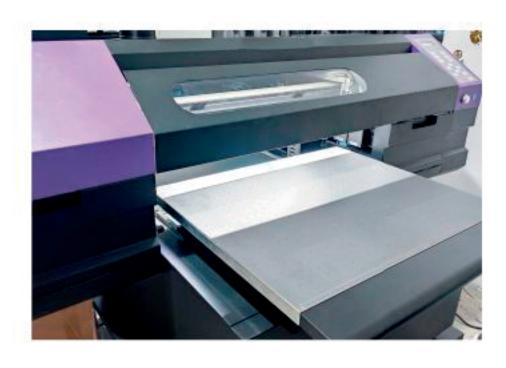
The overall printer cover can improve the operation safety, reduce the adhesion of dust in the printing process and ensure the printing quality.
